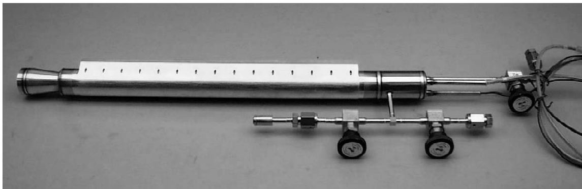
Fig. 4. Photograph of an assembled EBB compressor element with a ZrNi hydride gas gap actuator installed.
